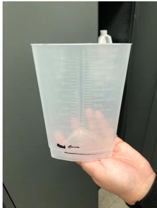
Photo 4: Using a graduated and marked measurement tool for mixing chemicals / disinfectants ensures the proper concentration is always reached.
